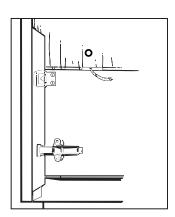
Failure to align the "V"s properly or to latch the drawer to the door may cause the compactor to not function properly.
